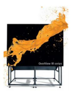
With the **OverView M** series, Barco enters the small- to medium-sized control room market, offering a DLP-based, SXGA (1400x1050) resolution monitor wall that includes 10-bit color processing and an 80,000-hour LED light source. The first range of OverView M video wall cubes to hit the market are the 4:3 aspect ratio versions, available with screen diagonals of 60", 67" and 80". Barco told rAVe that widescreen models will become available later this year.
