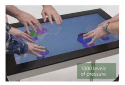
FlatFrog's **Planar Scatter Detection technology** (PSD) is the first multi-touch display technology to offer pressure detection.
