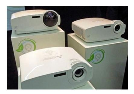
Mitsubishi Electric brings out the **LaserVue family of lamp-free projectors**, the company's first hybrid-design. To produce the red-green-blue lighting elements required to form all displays, Mitsubishi LaserVue projectors use one pure red LED and up to 34 pure blue laser diodes of varying strengths and wavelengths, and a solid-colored phosphor wheel that emits green light.
