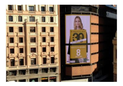
The installation at Callao measures 18.29 meters high by 10.61 meters wide and features SMD (Surface-Mount Device) technology at a 10 millimeter line spacing. The display includes a seamless angle that provides impressive viewing angles as it shows vibrant images with excellent contrast.
