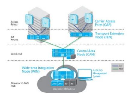
CommScope Era is **an all-digital C-RAN antenna system** that leverages wireless operators' initiatives to centralize and virtualize baseband radio assets, a foundational design concept for 5G networks.
