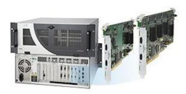
Extron Electronics is now shipping **HDMI Input and Output Cards** which add HDMI connectivity and HDCP compliance to the Extron Quantum Elite Videowall Processing System.
