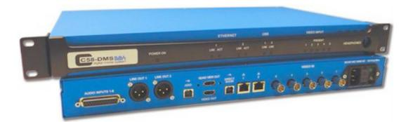
At InfoComm, PESA launched the **C58 Digital Media System** for recording, playback, and distribution of critical live video and audio content.
