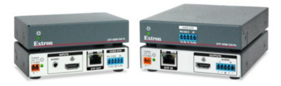
Extron Electronics announces immediate availability of the **DTP HDMI 230** twisted pair extender for transmission of HDMI, audio, and bidirectional RS-232 and IR control signals up to 230 feet (70 meters) over a single CAT 5-type cable.
